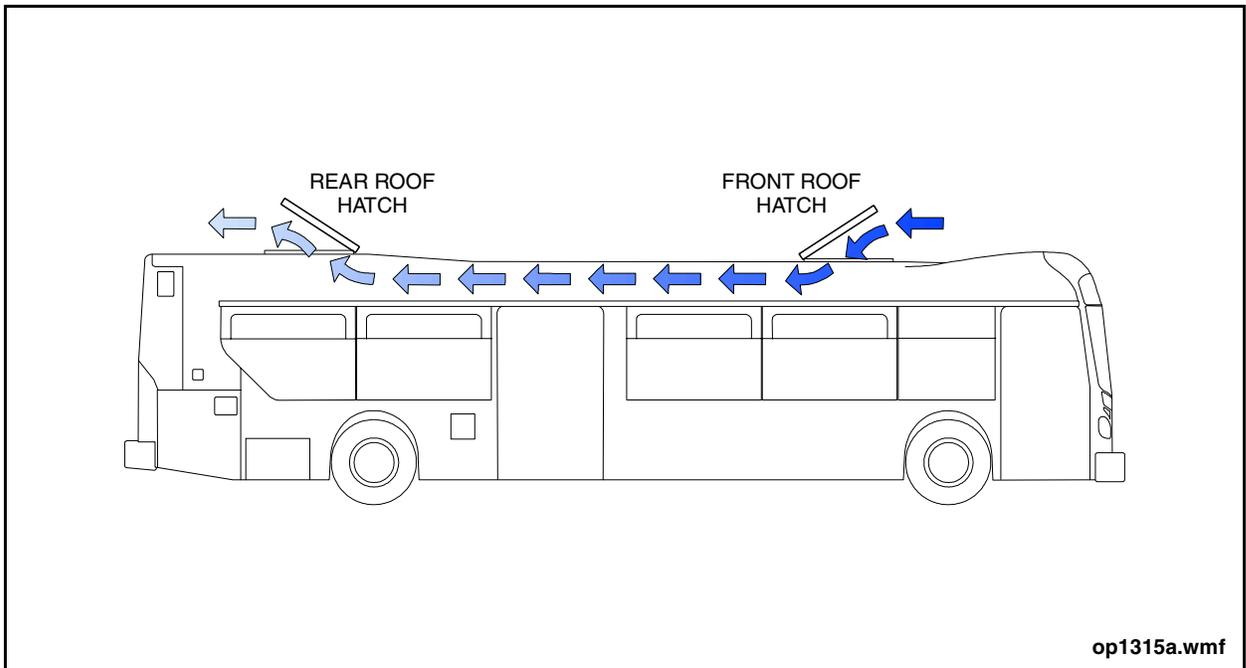
**Figure 34: Roof Hatch Ventilation**
