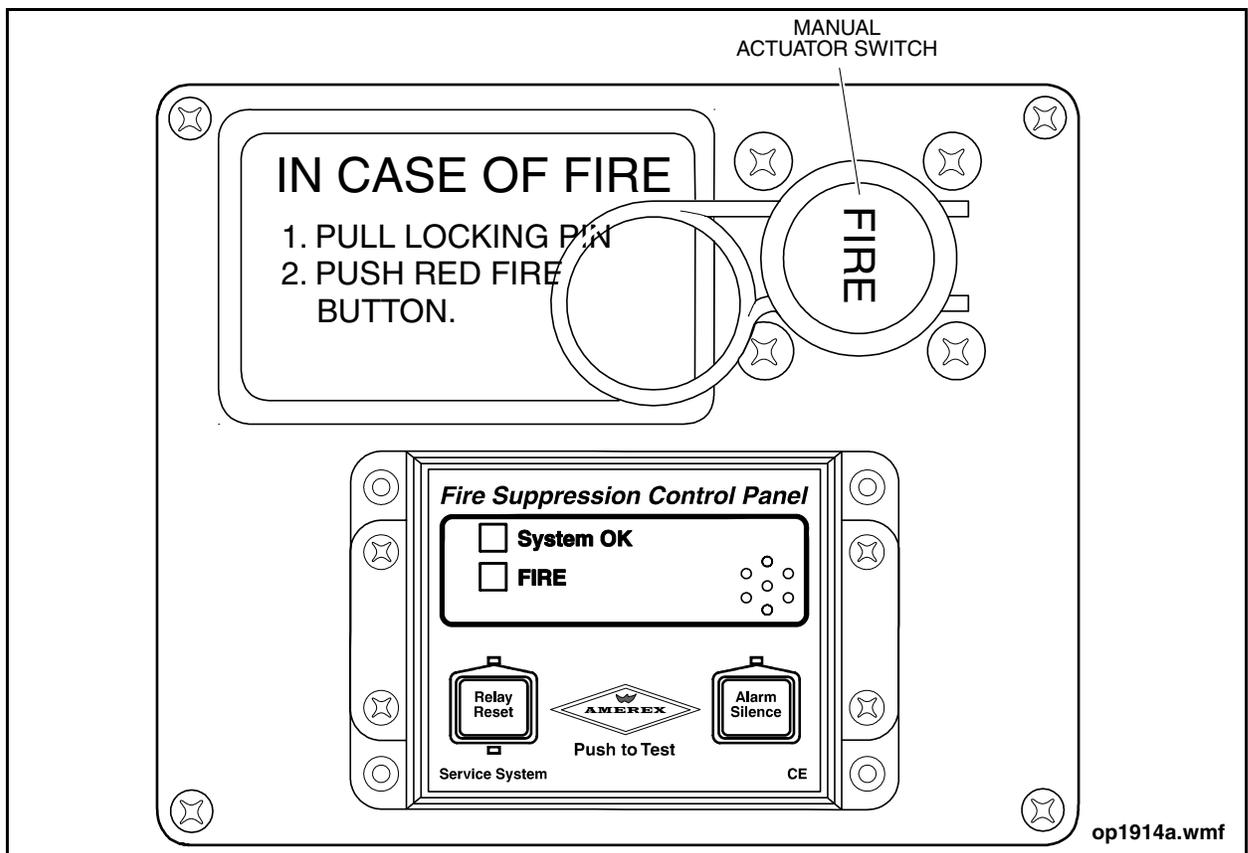
**Figure 31: Fire Suppression Control Panel & Manual Actuator Switch**
