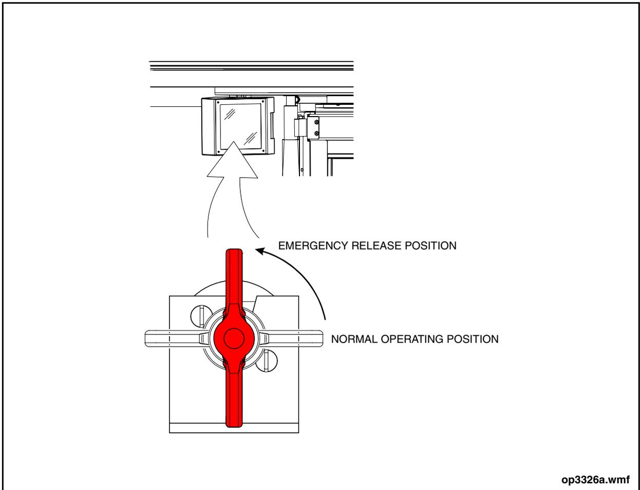
**Figure 5: Exit Door Emergency Release Control Valve**
