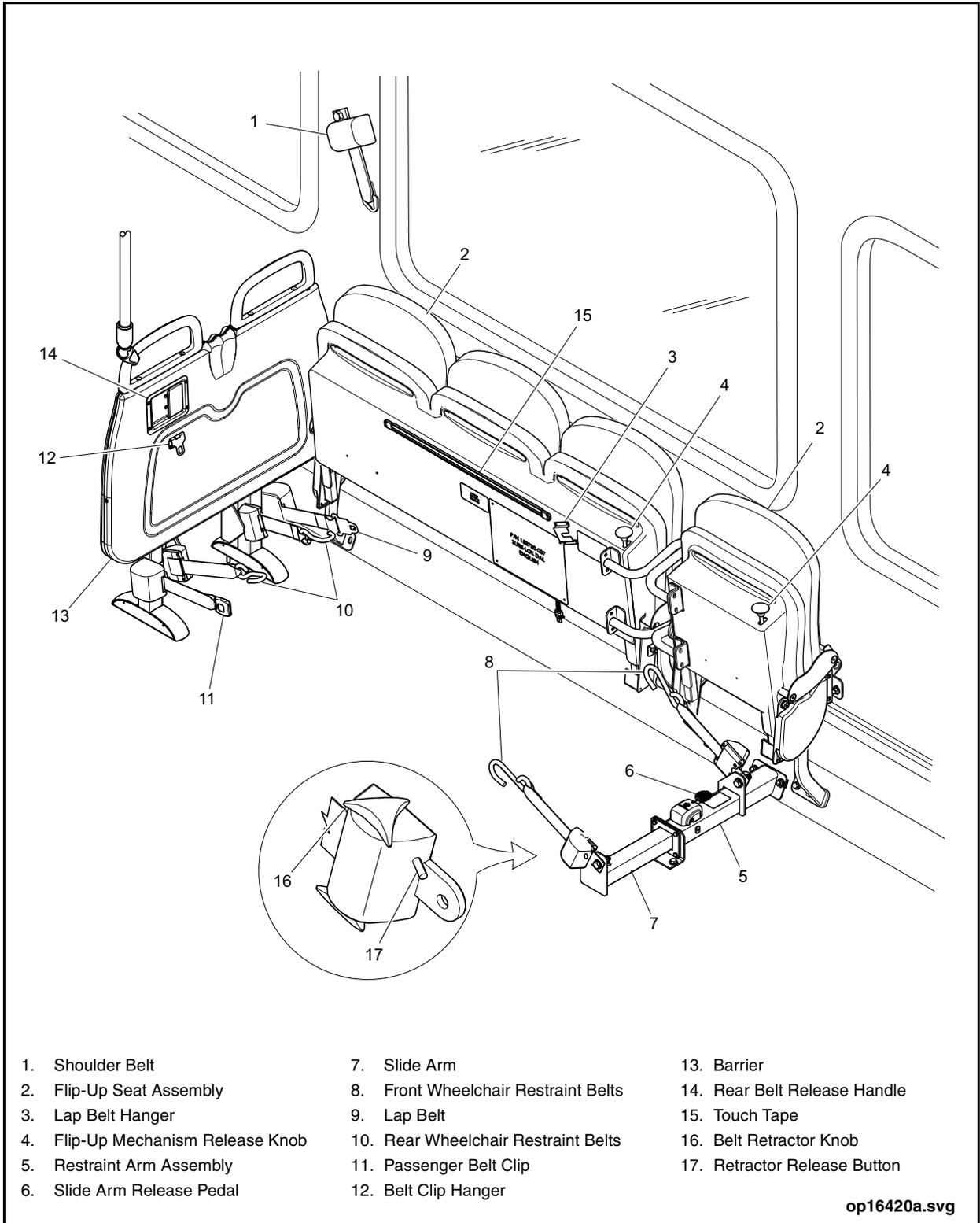
**Figure 36: Wheelchair Restraint System**
