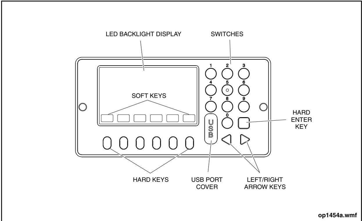
**Figure 19: Operator's Display Keyboard (ODK)**
