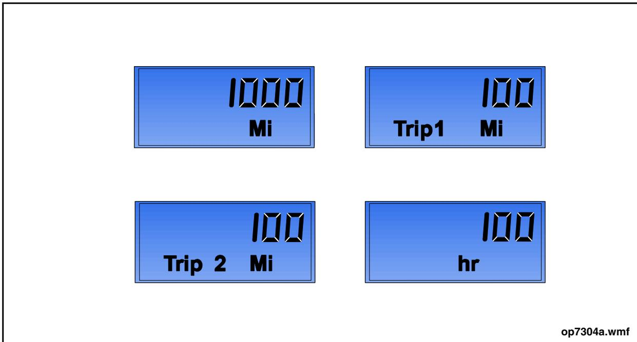
**Figure 24: Odometer/Hourmeter Display Screen Options**
