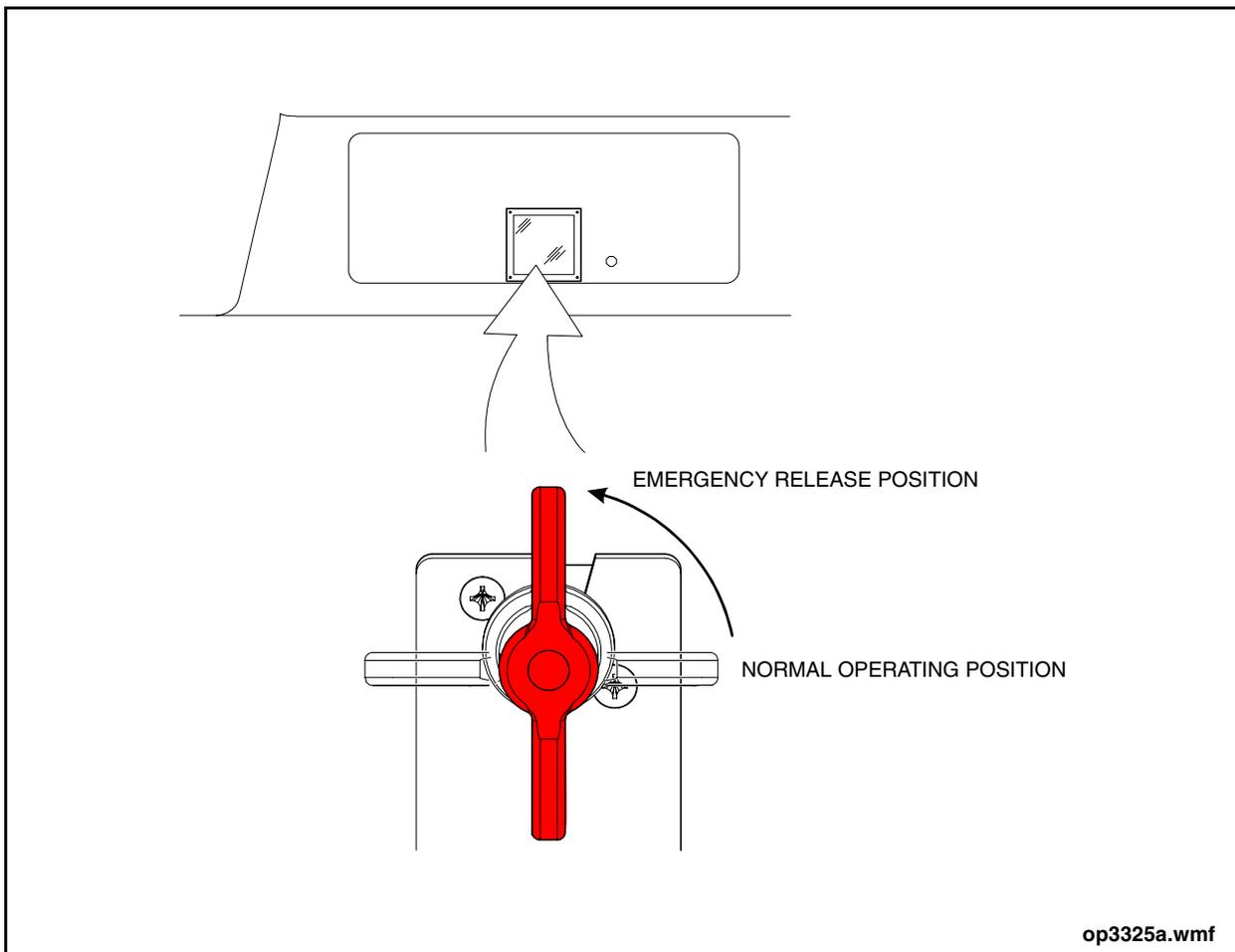
**Figure 4: Entrance Door Emergency Release Control Valve**
