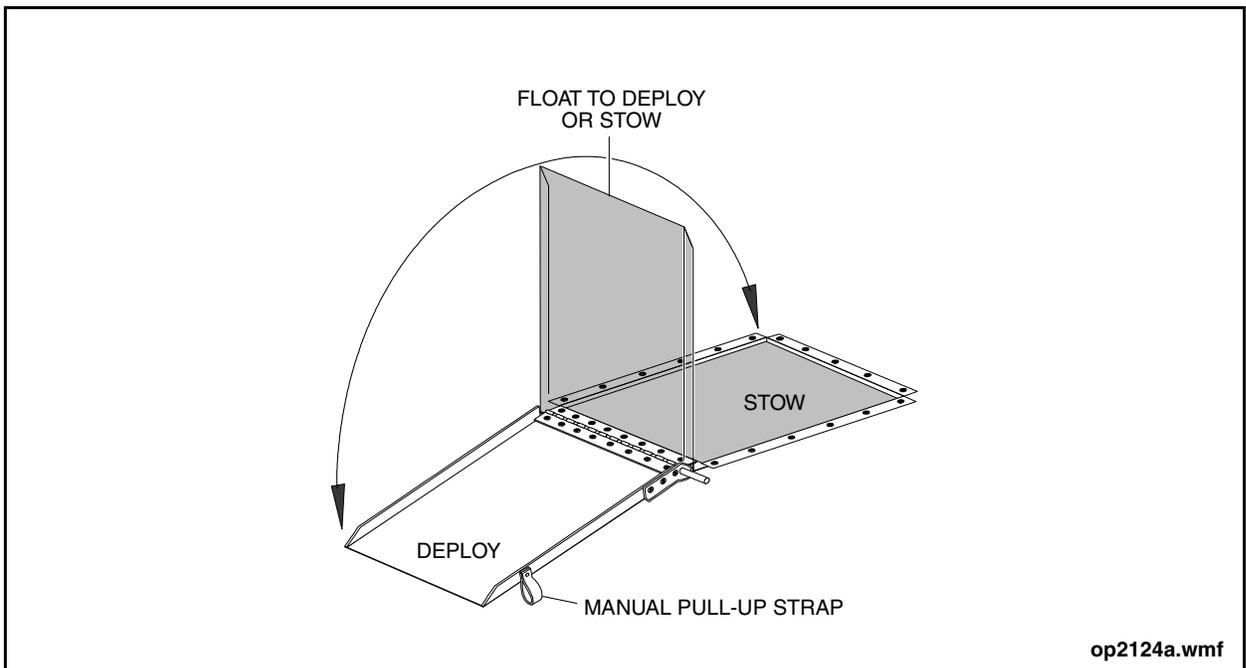
**Figure 35: Wheelchair Ramp Operation**
