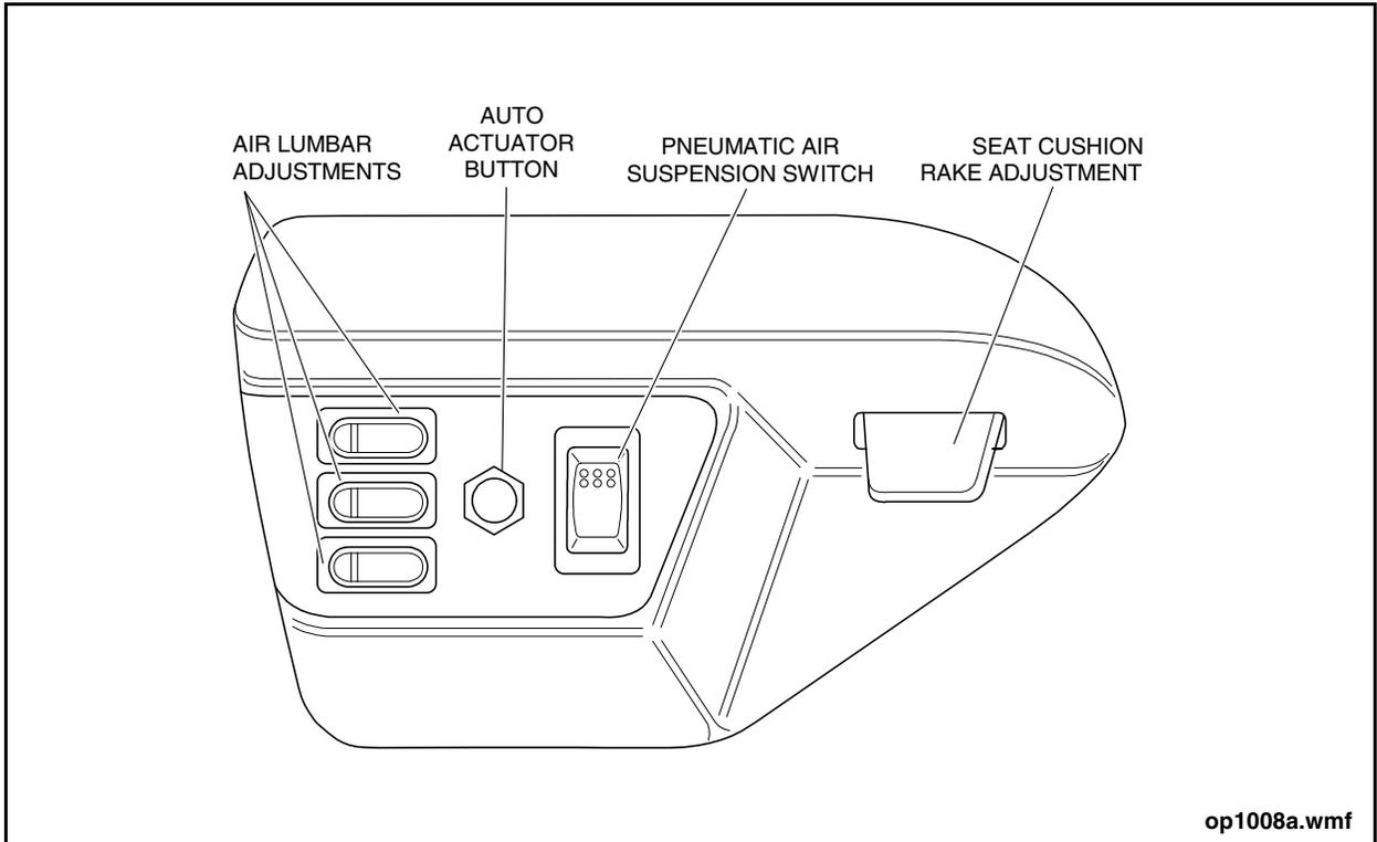
**Figure 15: Driver's Seat Switch Panel**
