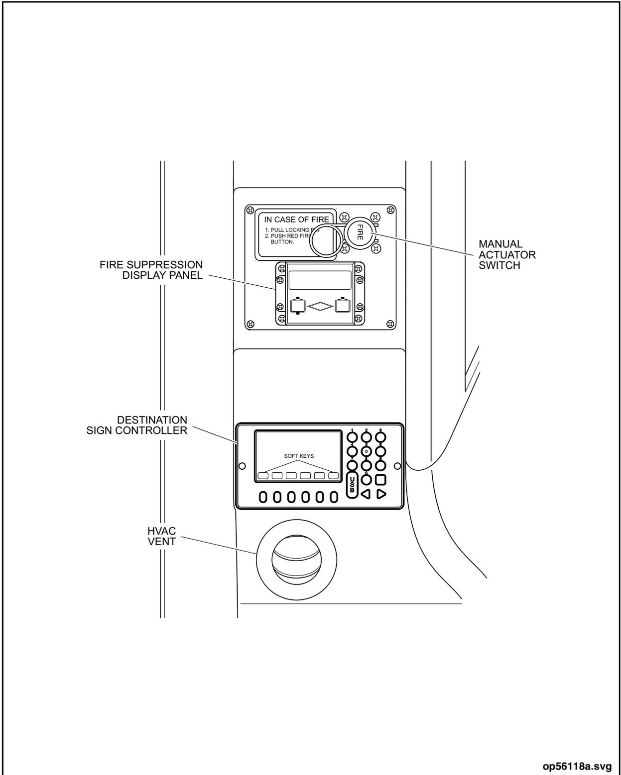
Figure 13: Driver's Overhead Panel
